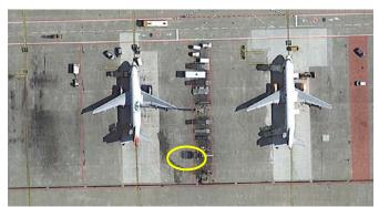
2. Do not position stairs just before the dotted line that outlines the way: stairs must be positioned inside the Equipment Parking Area (EPA) at least 3 metres away from Apron Border Line (ABL)
