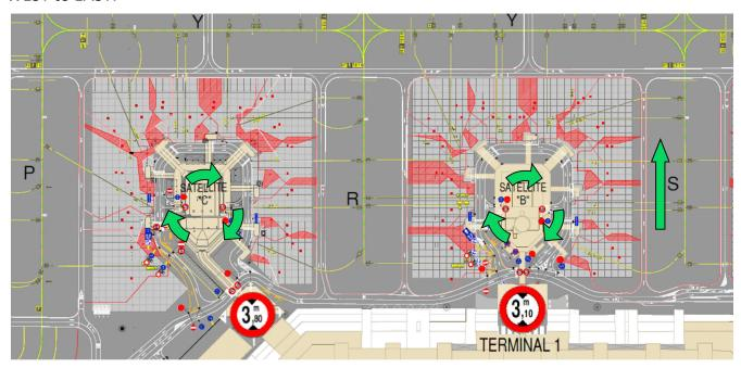
The possible critical issues for the vehicles' circulation along the NORTH/SOUTH/NORTH lines, parallel to the TWY Y, could be avoided by choosing the road closest to the terminal building, complying height and bearing capacity limits under connecting bridges to the Terminal 1 (Bravo e Charlie).
